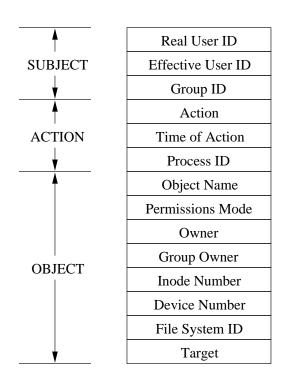
Figure 3.5: USTAT Audit Record Structure<sup>5</sup>
